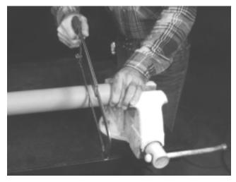
H. Using cut off section of shield as a guide, cut shaft the same amount. (Figure 2-4) Figure 2-4
